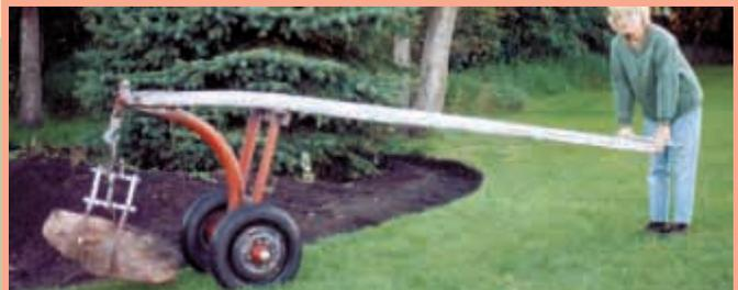
Manually-operated hand cart can be used to both lift and transport big rocks that weigh 300 lbs. or more.
