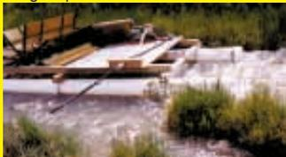
I've made improvements to the home-built floating paddle pump previously featured in FARM SHOW (Vol. 26, No. 6). The system uses the power of the flow-
