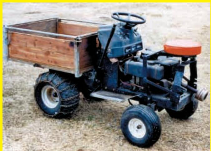
I made this wood hauler from an old riding lawn mower. The box trips to dump the wood. Works great and I can take it right
