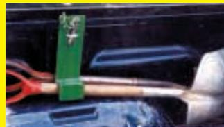
I came up with a nifty way to keep shovels and forks, in place in the bed of my pickup. The shovel handle lays across the wheel well and is held in place by a metal bracket. It keeps the shovel off the bed floor and out of the way. No drilling was required as I was able to use holes already in the bed. The bracket is secured by a tapered pin that goes through an I-bolt that's inserted through the side of the box. **(James Feldman, 10993 Stanton Blvd., Northfield, Minn. 55057)**
