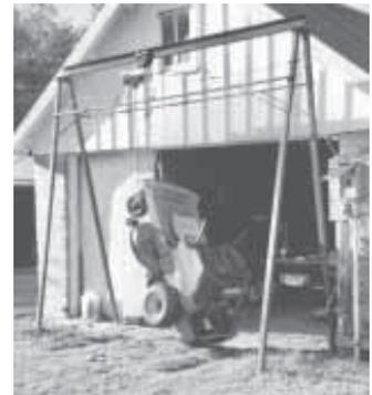
**Electric-operated hoist allows Hussong to raise his Snapper riding mower. It measures 12 ft. high and wide, with legs spread 4 ft. apart.**
