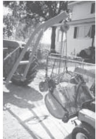
**Leonard Seltzer modified the hitch off an IH planter to build this "lift boom" that makes it easy to do maintenance work on his riding mower. A 1-ton chain hoist does the lifting.**
