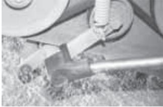
The baler's pickup is equipped with five or six bars, with grease fittings at both ends. To grease the bars, the operator has to either loosen the belt or remove it so he can rotate the pickup. The tool that Ellis fabricated simply takes the tension off an idler on the belt, allowing the operator to slip the belt off the pulley. The idler is attached by a short metal bracket to a shaft.
