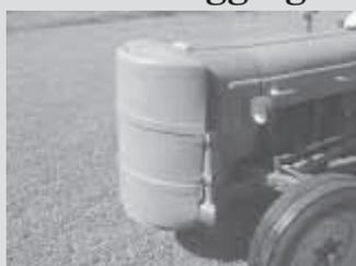
**Cut-up plastic barrel, wired to tractor's front grill guard, protects grill opening from flying debris.**
