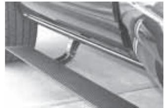
Retractable running board is activated by electric door sensors so it drops down and out in about a second when door opens.
