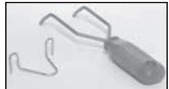
Two-pronged fork quickly wraps V-shaped clips around wire to hold it in place.
