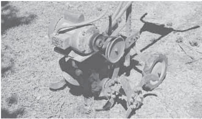
Electric motor, with pulley attached, bolts on in place of rototiller's original gas engine.
