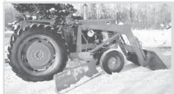
Hinged bracket allows 3-pt. snow blade to mount on side of Brandt's tractor.
