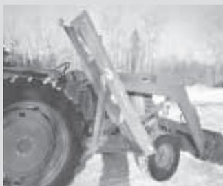
Steel cable runs from blade up through a pulley on side of tractor and out to bucket.
