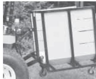
After unpinning the carrier from tractor, he can wheel it into his basement.
