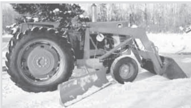
Hinged bracket allows 3-pt. snow blade to mount on side of Brandt's tractor.
