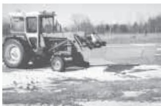
Ted Gaur a already had a blade on back of his Deere 2020 tractor. He put one on his loader as well, by converting a used truck plow. He put a piece of poly sheeting over it to keep snow from sticking.
