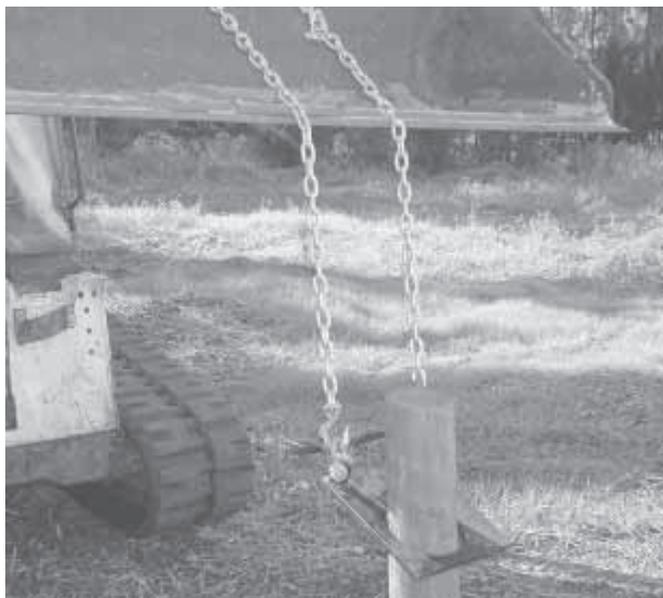
Large post-pulling plate pulls wood posts 3 1/2 to 6 in. in dia.
