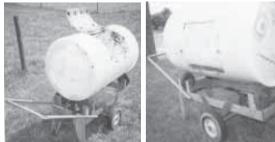
Composter rides on a 2-wheel trailer with a handle on front so it can be pulled around by hand. Barrel rotates on four riding lawn mower wheels.
