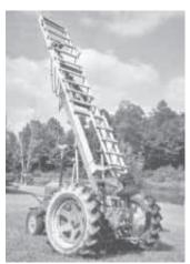
Homemade ladder is 21 ft. long when extended. It attaches to tractor's boom with
