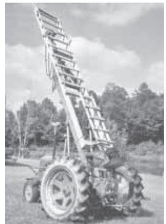
Homemade ladder is 21 ft. long when extended. It attaches to tractor's boom with U-bolts.
