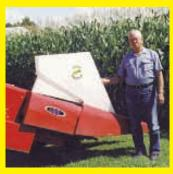
No. 6). The triangular-shaped attachments bolt to each side of the header and deflect ears back onto the snouts, saving 3 to 5 bu. per acre even under normal conditions.
