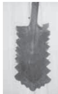
**Bill Reeks modified a conventional pointed shovel by cutting "teeth" into the sides and bottom of it.**
