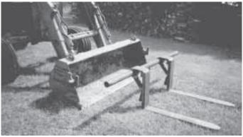
Kenneth Aller, Louisville, Ohio: "For years we handled material on pallets by hand. We needed an easier, inexpensive way to do the job so we decided to use the loader bucket on our Deere 2555 tractor. We welded a bracket onto each side of the bucket, then mounted a set of forks onto a length of steel
