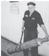
works especially well on cylindrical gas tanks. It also works great for carrying metal or plastic pipe that's wet or muddy because the belt won't slip like my hands might. Serpentine belts can be found on most late model cars and trucks. I've used this idea for 10 years. Before serpentine belts came along I used conventional V-belts."
