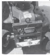
of it that allows me to lift the front end of the tractor. As a result, I can sharpen blades without having to remove the tractor's 42-in. mower deck or reach underneath it. I place a safety stand under the deck so it can't fall.
