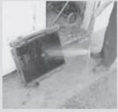
Homemade tool allows Wasson to clean out a radiator while it's still on the wehicle.
