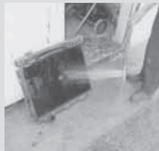
**Homemade tool allows Wasson to clean out a radiator while it's still on the vehicle.**
