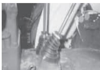
They didn't quite fit watertight so I used two stainless steel clamps to secure them to the gear shifter. The best part is I didn't spend more than \$15.
