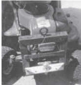
of it that allows me to lift the front end of the tractor. As a result, I can sharpen blades without having to remove the tractor's 42-in. mower deck or reach underneath it. I place a safety stand under the deck so it can't fall.
