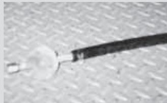
**Tool consists of a 30-in. long piece of flexible 3/8-in. hydraulic hose, with a 2 1/2-in. long piece of copper water pipe at one end. A large washer welds to pipe**
