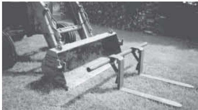
**Kenneth Aller, Louisville, Ohio:** "For years we handled material on pallets by hand. We needed an easier, inexpensive way to do the job so we decided to use the loader bucket on our Deere 2555 tractor. We welded a bracket onto each side of the bucket, then mounted a set of forks onto a length of steel
