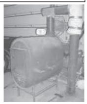
side of the fan and filters the air before it goes through the fan motor. I lined both sides of the stove with fire brick and also welded a couple of angle iron stiffeners lengthwise to both sides of the stove to keep the sides of the barrel from buckling. The stiffeners are spaced 6 in. apart and located just above the fire brick.
