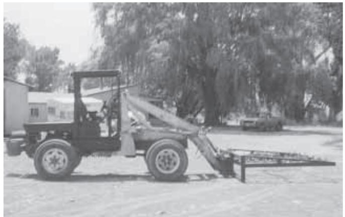
Loader picks up 18 two-wire bales at a time, allowing him to load a semi in minutes.
