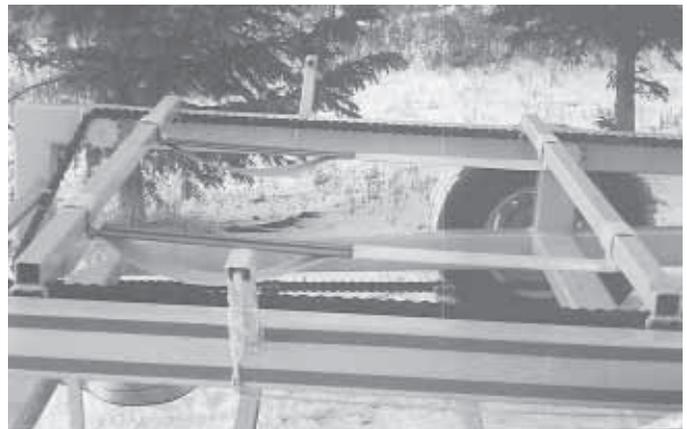
As a bale is pushed onto the trailer, it falls between two cross bars and onto two 4-in. wide straps that cradle the bale.
