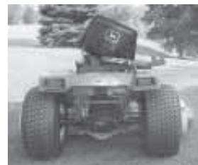
Andy Justmann modified the seat on his Deere garden tractor so that it can be tilted 35 degrees in either direction. A single hydraulic cylinder tilts the seat.
