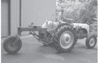
Lee deVries uses this home-built, 3-pt. mounted dolly to put his fifth wheel trailer into storage. Dolly takes much of trailer's hitch weight off tractor's 3-pt. hitch.
