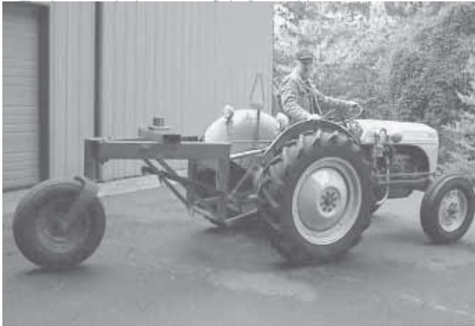
Lee deVries uses this home-built, 3-pt. mounted dolly to put his fifth wheel trailer into storage. Dolly takes much of trailer's hitch weight off tractor's 3-pt. hitch.
