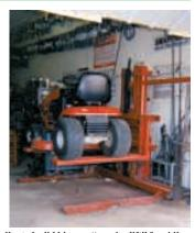
Rissler used an old forklift mast and hydraulics to build his own "service lift" for riding mowers. Mower's front and rear wheels rest between two lengths of tubing.
