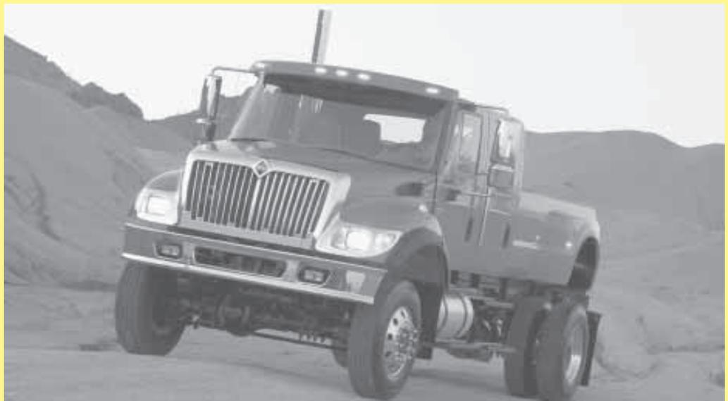
**Big Red pickup was put together by an International Truck dealer in Arizona. The base truck comes standard with full-time 4-WD and is powered by a 215 hp diesel engine. Big chrome stack and bright metal work make it somewhat resemble a semi tractor.**
