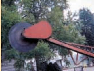
The 30-in. buzz saw mounts on the end of a 20-ft. length of steel tubing. "The saw is far enough in front of the loader that I don't have to worry about branches falling on me," says Brenneman.
