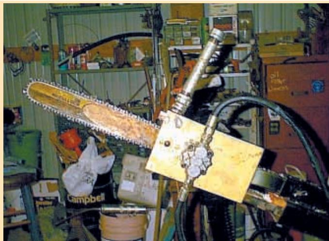
Pipe filled with lubricant keeps chain from getting too hot during hard cuts.
