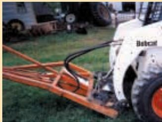
Saw is belt-driven by a hydraulic motor that operates off skid loader hydraulics.
