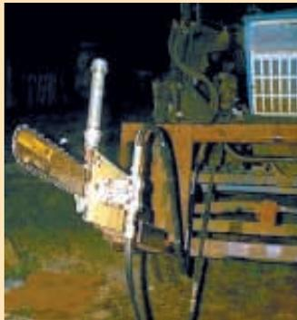
Hydraulic-powered chain saw slips on and off the forks on Ronnie Campbell's front-end loader.
