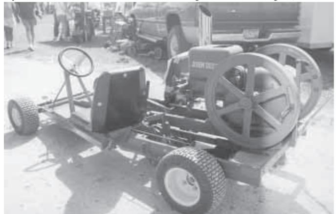
Engine rotates in the opposite direction as go-cart's main driveshaft. Deschene used a couple of belt pulleys and shafts to reverse the drive.
