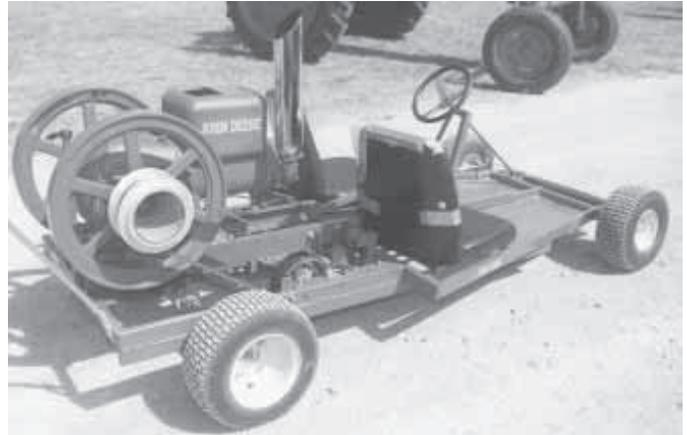
“When it fires it sounds almost like a shotgun going off,” says Jack Deschene, who built this go-cart that's powered by an old 3 hp Deere E “hit and miss” gas engine.
