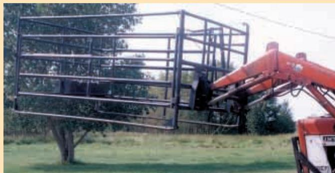
Cage mounts on any loader equipped with quick-tach bucket mounts.
