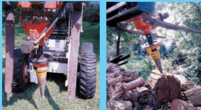
He also removed post hole digger's pto shaft and added a hydraulic motor (left). No wood is too big or too hard to split, says Hathaway.
