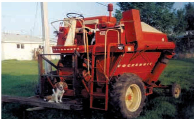
Converted combine hauls grain in hopper and bales on 3-pt. hitch bale forks that mount in place of header.
