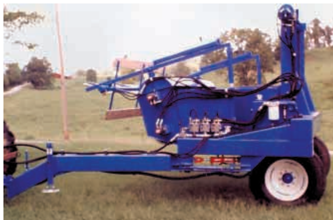
Wild grass seed harvester boasts a 90 to 95 percent seed recovery, even in rougher, rolling terrain, says the manufacturer.
