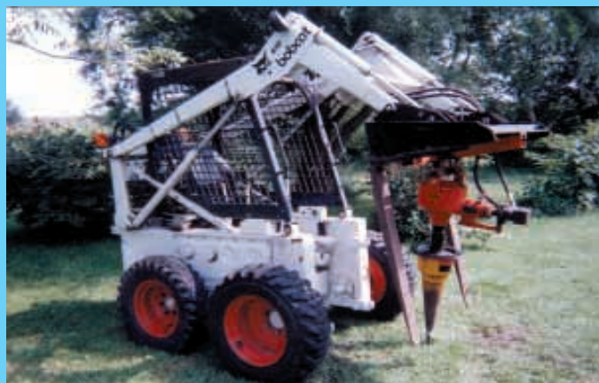
John Hathaway hooked up a Stickler screw-type wood splitter to an old 3-pt. posthole digger, which he modified to fit the loader arms on his Bobcat skid steer loader.
