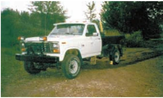
Converted pickup lets Steve Prins haul small amounts of gravel and blade it down with the same machine.
