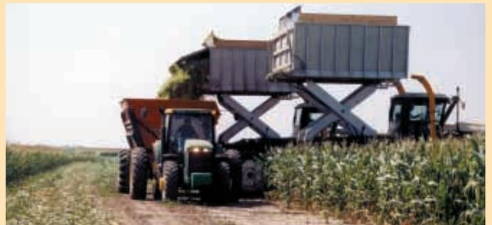
High-lift hoppers mount on scissor-hoists that can easily dump into a semi trailer or dump cart.
