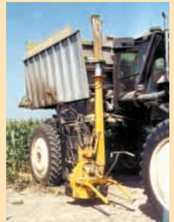
Hydraulic-powered choppers blow silage into hoppers on back of machine.
