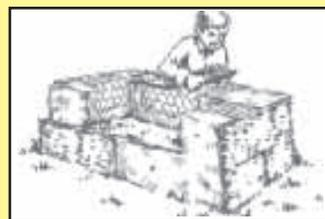
Stakes form outline of sofa (above left). Waferboard forms a mold that's filled with dirt (above). Sod laid over chicken wire is held in place with planting stakes (left).
