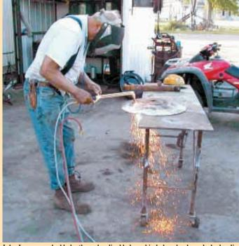
John Jensen punched holes through a disc blade, a chisel plow shank, and a hydraulic cylinder shaft in the course of testing this new gasoline-power ed torch.
