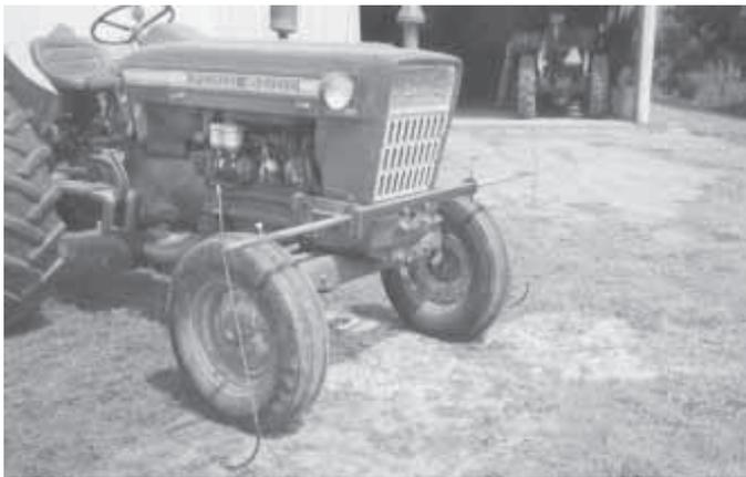
Rods at ends of crossbar are fitted with lengths of rubber tubing that follow the row.
