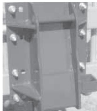
Quick-tach bracket attaches to any tractor or skid steer.
