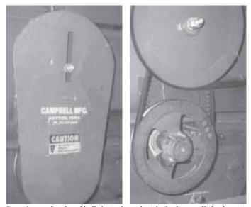
Straw chopper slow-down kit eliminates the need to take the chopper off when harvest-ing corn and also extends chopper life. Unit spreads corn residue safely by limiting the distance and speed that it's thrown out.
