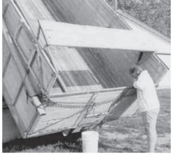
Robert Bokenfohr modified the top half of his truck box endgate so that he can flip it up and out of the way. It's no problem to reach in while standing at the back of the box to scrape out the corners.
