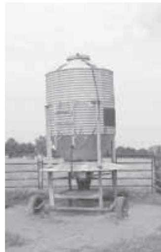
Bud Wright removed the top two rings from a 10-ton feed bin and then turned it into a nifty portable feeder. He welded two of the bin's four legs to the axle and wheels off an old trailer.
