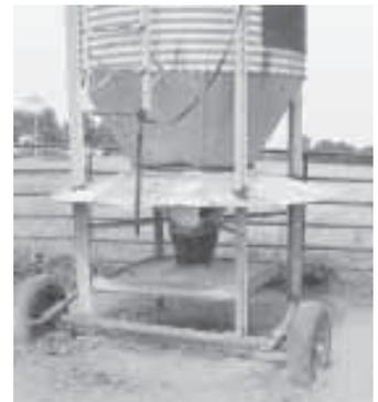
A 4-ft. sq. "swinging" wooden platform mounts between the legs. Feed gravity flows out of a manually-operated slide gate at bottom of bin.
