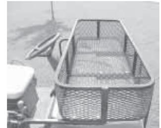
Front basket is used for carrying supplies and tools (above). He also mounted a two-piece receiver hitch on back of his Gator (below).
