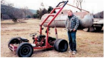
"It can be used to move almost any heavy object," says Bob Unger about his self-propelled "boom loader." The 2-WD rig is powered by a 5 hp Briggs & Stratton engine.
