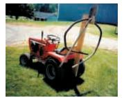
Wooden rack mounts on back of tractor and is used to carry a shovel as well as the hot exhaust pipe.
