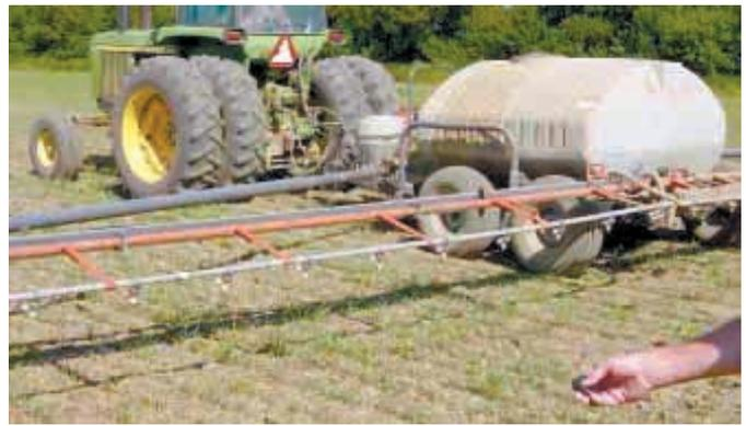
Remote controlled boom lets Dale Wiens stand behind his 90-ft. sprayer and turn each boom section on and off individually to make sure nozzles are working properly.
