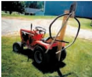
Wooden rack mounts on back of tractor and is used to carry a shovel as well as the hot exhaust pipe.
