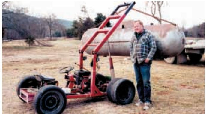
"It can be used to move almost any heavy object," says Bob Unger about his self-propelled "boom loader." The 2-WD rig is powered by a 5 hp Briggs & Stratton engine.
