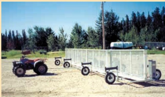
Field-size bug zapper consists of a 20-ft. wide by 4-ft. high steel mesh center panel, with a 10 by 4-ft. wing on each side. Each panel has three electrified grids.
