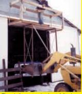
The platform stands about 9 ft. above the loader bucket and measures 10 1/2 by 3 ft. 1 in. The entire structure is made from used 2 by 8 lumber, angle iron, pipe and silo rods. The unit attaches to the bucket with five bolts and can be easily removed for storage. A safety railing around the top can be removed by lifting four pins at the corners. (*Jim Feldman*, 10993 Stanton Blvd., Northfield, Minn. 55057 ph 507 645-8771)
