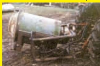
company where I work. I cut it up to make a drum and then mounted a ball fin inside it that I made out of an old grinder. An orbit motor is used to chain-drive a rubber
