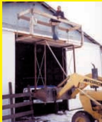
The platform stands about 9 ft. above the loader bucket and measures 10 1/2 by 3 ft. 1 in. The entire structure is made from used 2 by 8 lumber, angle iron, pipe and silo rods. The unit attaches to the bucket with five bolts and can be easily removed for storage. A safety railing around the top can be removed by lifting four pins at the corners. (**Jim Feldman, 10993 Stanton Blvd., Northfield, Minn. 55057 ph 507 645-8771**)
