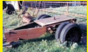
soft ground the pickup didn't have enough traction. To solve the problem, I built this fifth wheel hitch dolly that lets me use my tractor to pull the trailer. I bolted a ball onto a big steel plate and then welded the plate onto a truck axle, which is equipped with dual wheels. (**Steve Devaney, 7312 County Road 454, Merkel, Texas 79536 ph 915 537-2303**)
