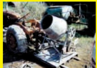
a pto driveline that runs under the mixer. The driveline has a pulley at one end. If I want I can mix cement on the way to the job, just like a cement mixing truck does. It comes in handy for pouring cement around posts when building fences. When unloading, the cement falls onto a piece of tin roofing mounted at an angle on one side of the pallet. It saves a lot of wheelbarrow work.
