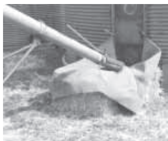
Three straw bales and a piece of old carpet - that's all Dean Nixon needed to make an auger hopper that he says works better than anything he could buy.
