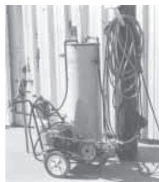
**George (Bing) Ribble converted a used power unit from a commercial car wash into this portable pressure washer. When he needs hot water to wash, he hooks it up to a 40-gal. gas water heater that stands next outside his shop building.**
