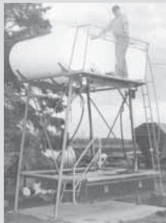
**Fuel tank stand holds three 300-gal. tanks 9 ft. off the ground and has a two-step ladder and handrail.**
