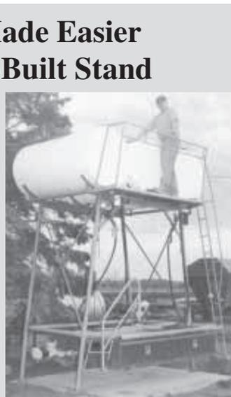
**Fuel tank stand holds three 300-gal. tanks 9 ft. off the ground and has a two-step ladder and handrail.**
