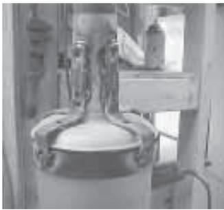
**Ken Sharabok, Waverly, Tenn.:** "Bushhogging is hard on a muffler. If a limb doesn't reach out and knock it around, the back and forth jarring tends to weaken or break the weld at the bottom. When I put a new muffler on recently, I made a bracket out of strap metal and angle brackets. The welding is kind of ugly but it's strong. (Muffler is upside down in photo.)"
