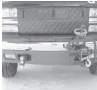
Standard 2-in. front receiver hitch bolts on in place of factory tow hook. If desired, a removeable winch can be mounted on either hitch (right).
