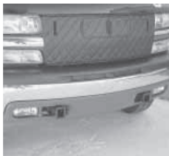
Standard 2-in. front receiver hitch bolts on in place of factory tow hook. If desired, a removeable winch can be mounted on either hitch (right).
