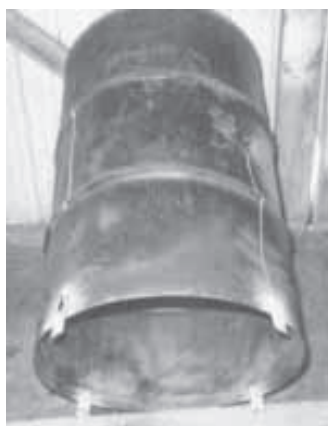
After removing both ends of 55-gal. drum, Prebble bolted four legs to bottom rim. Legs elevate barrel about 2 in. off the ground, creating a chimney effect.
