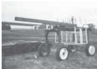
This is what the corn detasseling machine originally looked like before Litchfield made the conversion.
