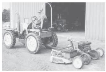
Marshall Litchfield converted an old detasseling machine into a small, 4-WD hydrostatic drive tractor. It's shown here pulling a big home-built lawn mower.
